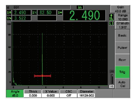
Figure 10-19 Verifying the refracted angle
