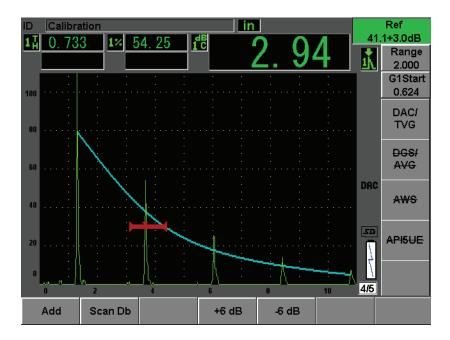
Figure 12-9 ASME DAC with 3 dB scanning gain
