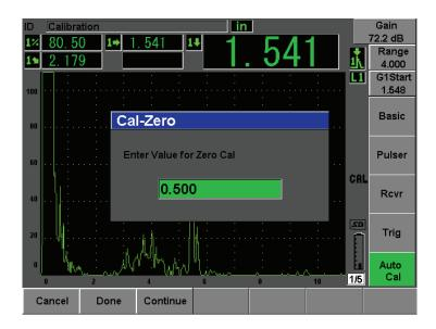
Figure 10-27 Entering the Zero Cal thickness value
