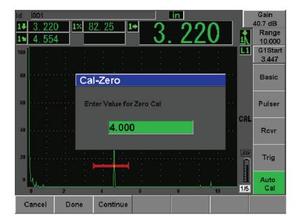
Figure 10-21 Entering the Zero Cal thickness value
