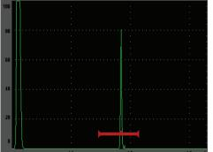
Leg grid: displaying vertical lines representing angle beam inspection legs. This mode displays up to 4 divisions, labeled L1 to L4, which represent each half-skip distance of a test piece during an angle beam inspection. The spacing and number of divisions displayed depends on the Basic > Range, Basic > **Delay**, and **Trig > Thick** (material thickness) parameters.
