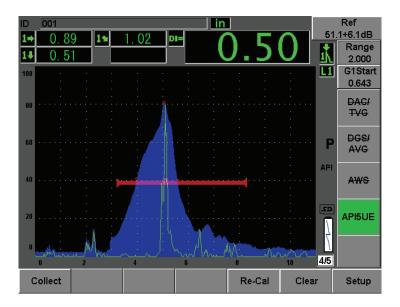
Figure 12-21 Completed API 5UE sizing
