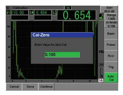
Figure 10-11 Entering the Zero Cal thickness value
